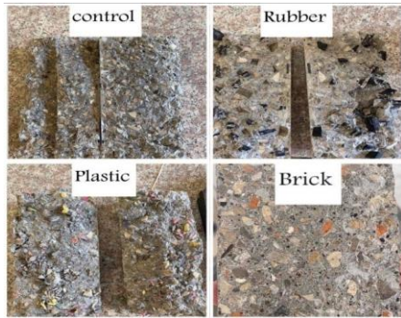
Fig. 15: Failure pattern of concrete containing different type of waste materials in splitting tensile strength.
