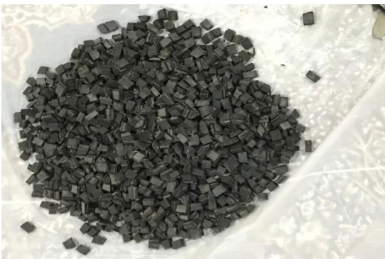
Fig. 3: View of crumbed rubber particles.
