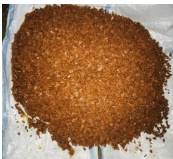
Fig. 5: View of crushed brick particles.
